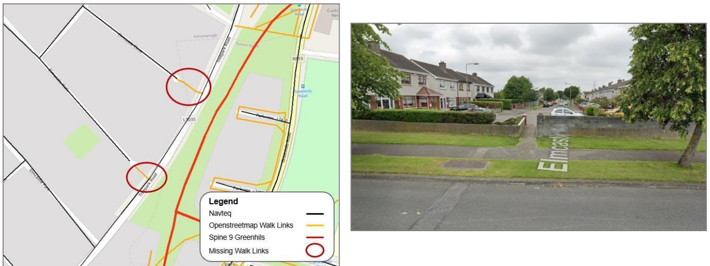
Figure 4.2 Example of permeability link missing from Navteq mapping on Tallaght/Clondalkin Cor Bus Corridor.
