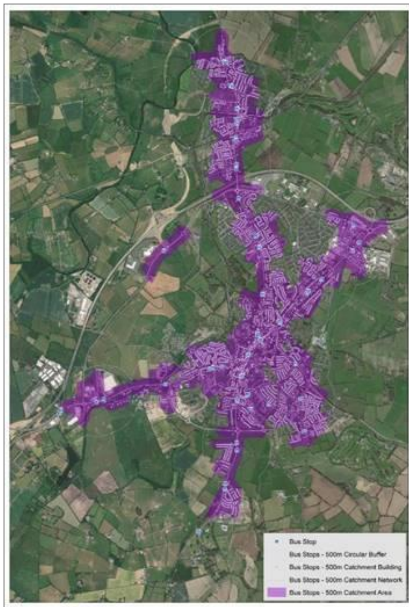
Figure 4.3 Example of catchment analysis run for all bus stops in Naas
